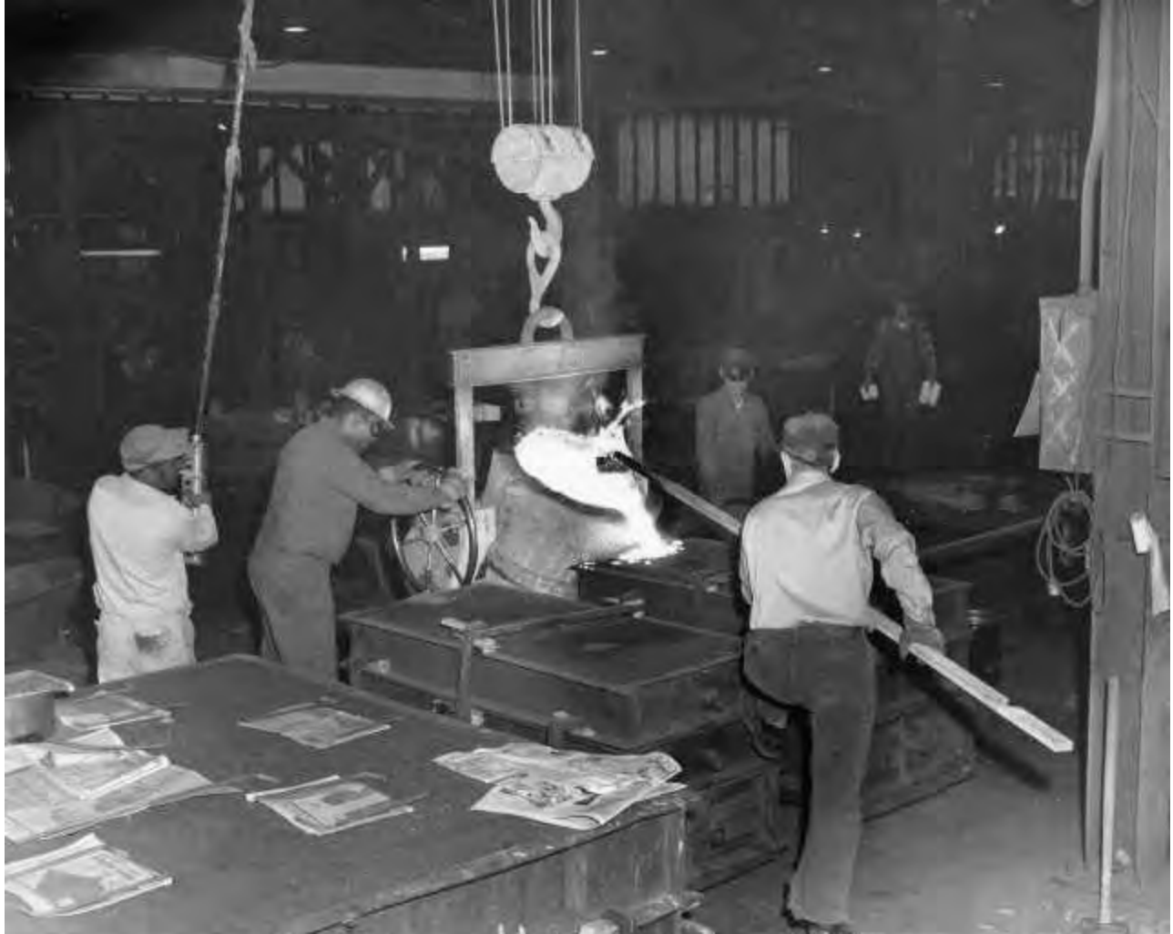
Molten liquid is being poured into molds at Fick Foundry, 1005 East D Street, in October of 1969. In business since 1924, Fick Foundry were producers of "quality static and centrifugal castings in most ferrous metals, and close tolerance aluminum centrifugal castings." The company had suffered through three major fires and was rebuilt each time. It would finally close in the late 1980's.
