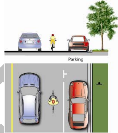
Example of On-Street Parking Delineation
