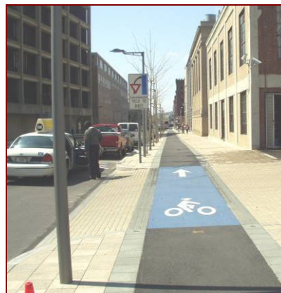
This cycle track in Cambridge, MA is separated from traffic by parking, light poles and grade
