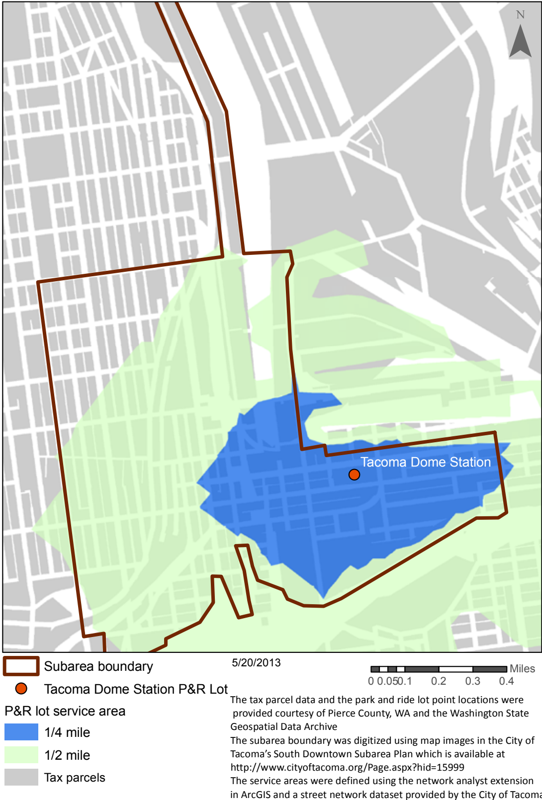
Figure 4: Pedestrian service area for the Tacoma Dome parking structure
