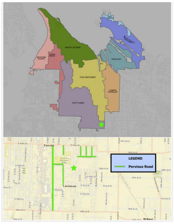
The Larchmont Permeable Neighborhood Project will improve water quality in the Flett Creek Watershed through replacement of approximately 27 blocks of failed residential roadway with permeable pavement. This project will provide basic treatment of stormwater for common urban contaminants and will also reduce flows through stormwater infiltration. The project will provide 43 acres of water quality treatment and increased flow control to help restore natural hydrologic conditions in this basin.
