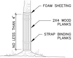
Install 2-inch thick wood planks around the trunk of the tree with 1/4" or greater closed-cell foam pads between the trunk and planks. The height of the wood planks shall be 4 feet minimum, or match the height of the vehicle clearance, whichever is greater. Use straps or wire to bind the planks in place. DO NOT drive fasteners into the tree. If the protective planks are to be in place for longer than 6 months, loosen and adjust the planks every 3 months to allow for growth.
