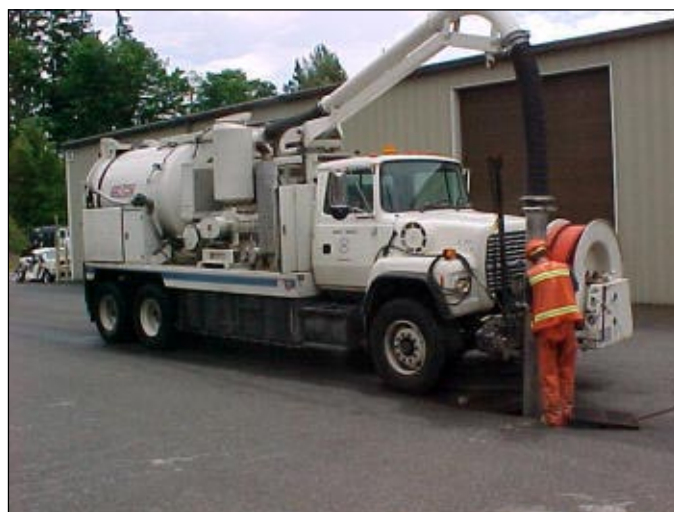
Vactor truck removing sediment from catch basin
