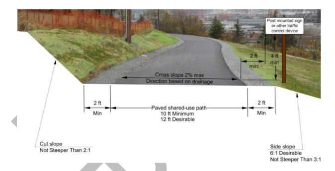
Figure 11-2: Two-way Shared-Use Path: Adjacent to Roadway (≤ 35mph)
