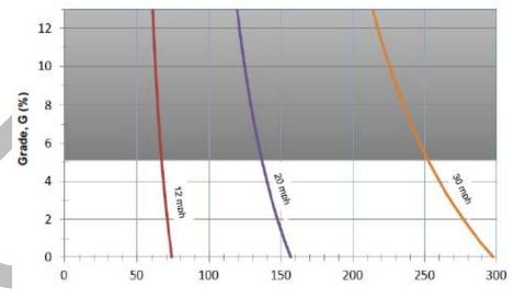
Stopping Sight Distance, S (ft) (Based on 2.5 second reaction time)
