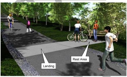
Figure 11-6: Landing and Rest Area Example
