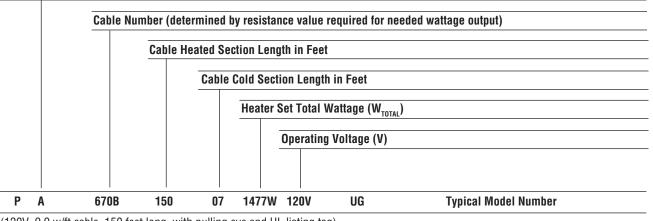
(120V, 9.9 w/ft cable, 150 feet long, with pulling eye and UL listing tag)
