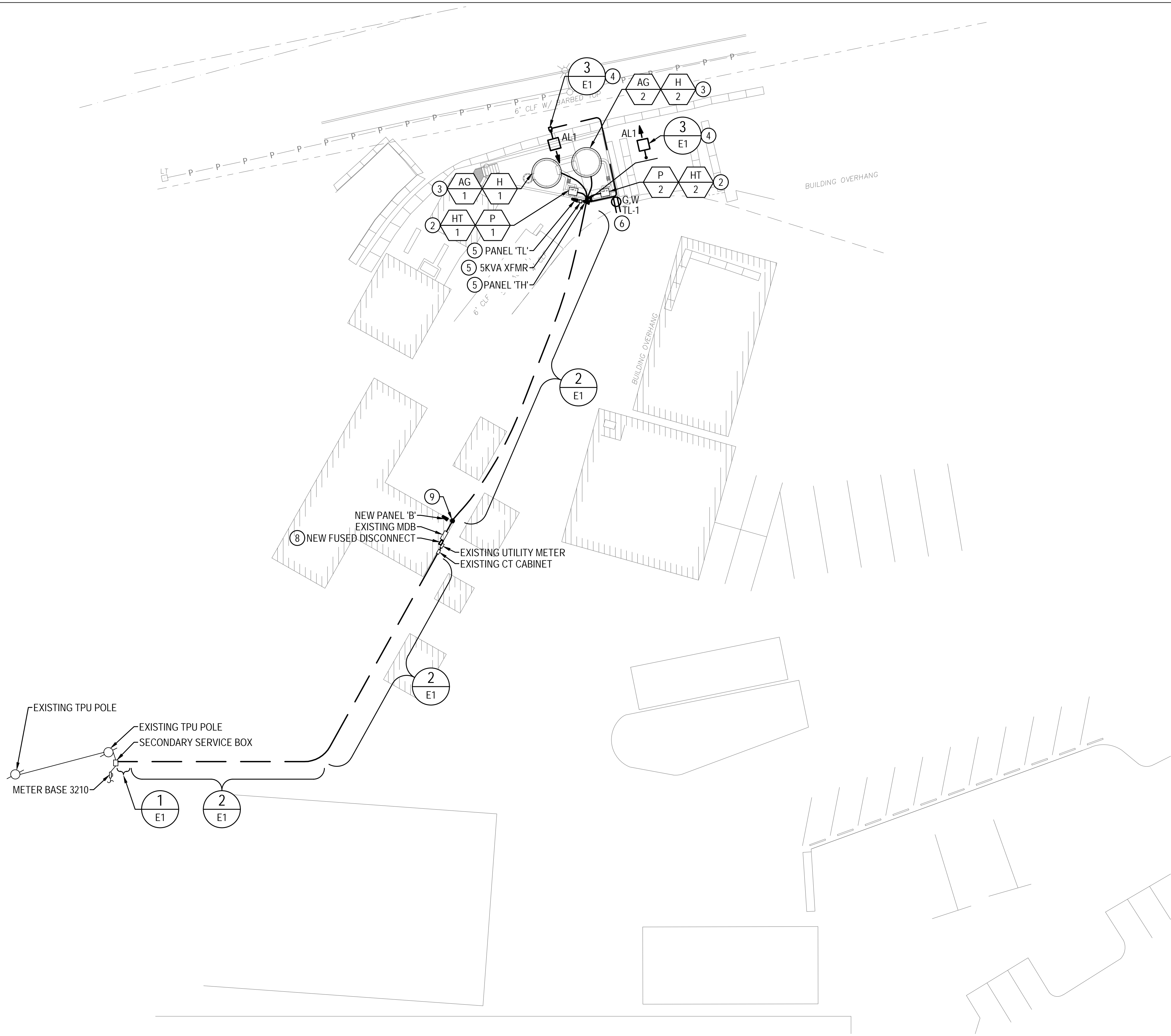
ELECTRICAL SITE PLAN 1 SCALE: 1" = 20'-0"
