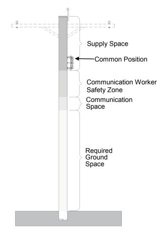
Figure 2 Illustration of Communication Worker Safety Zone
