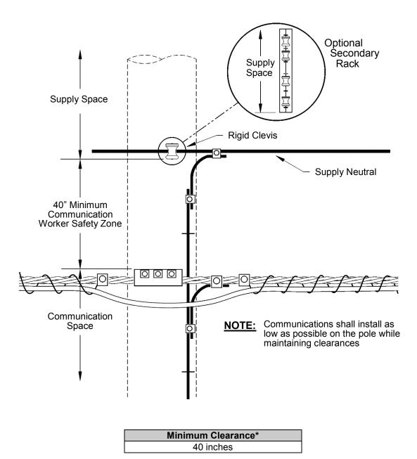
The minimum clearance may be reduced to 30 inches on a per structure basis as reviewed and approved by the Tacoma Power Line Section.
