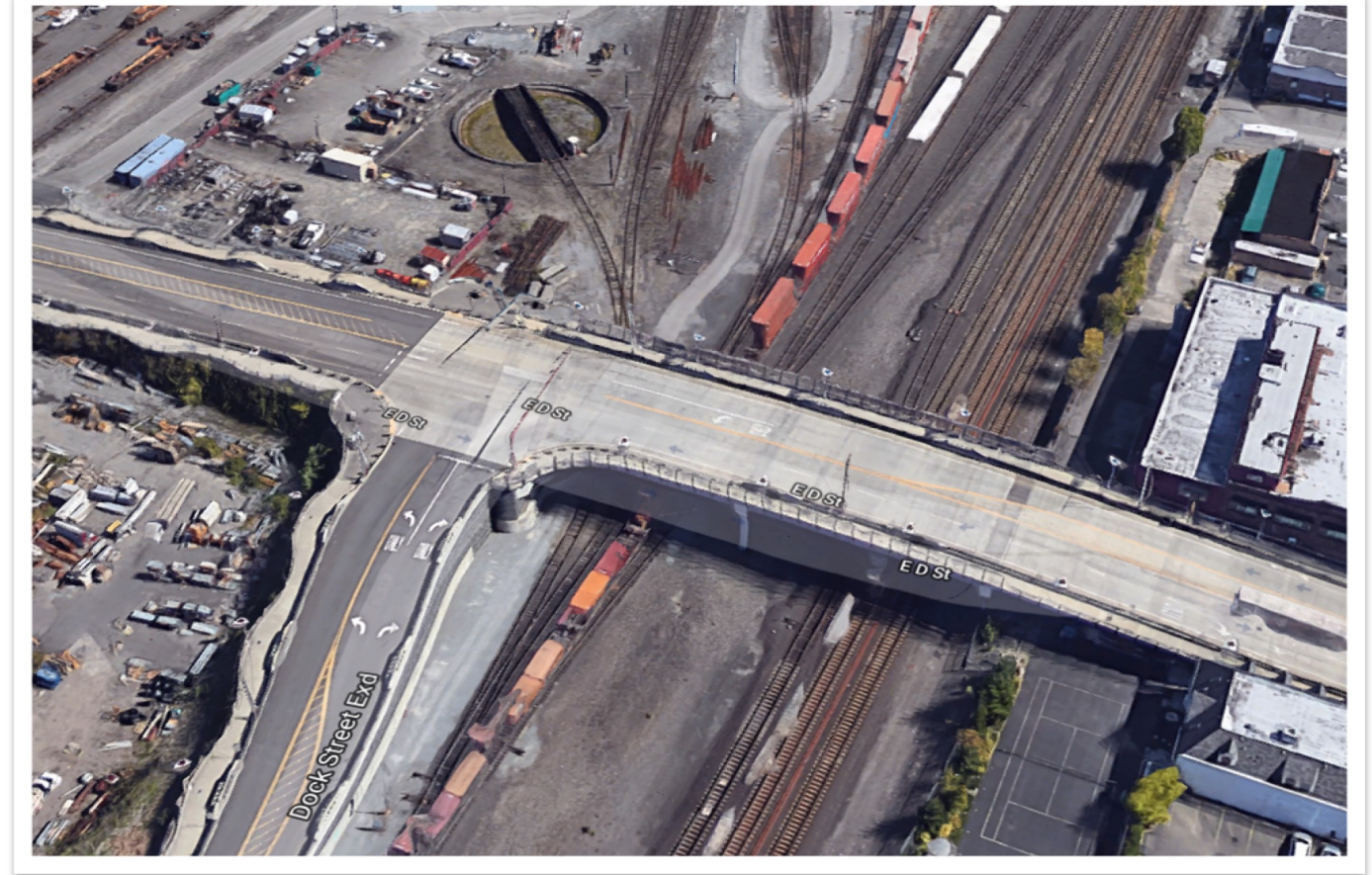
Example of a full grade separation.
