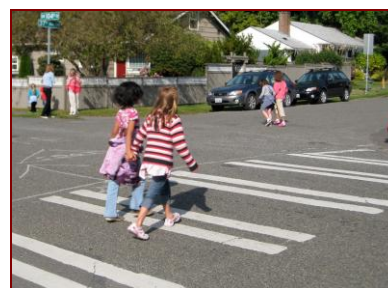
European type crossings (also known as 'piano' style) are one of the standard crosswalk designs in Tacoma
