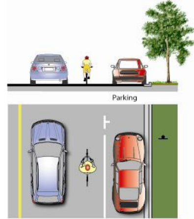
Example of On-Street Parking Delineation
