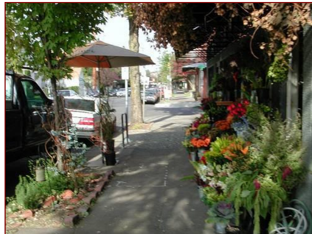
This sidewalk has plantings in the furnishing zone and in the frontage zone, and also provides sufficient through passage zone width
